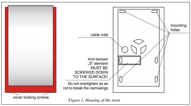
After installation of the siren, it is recommended that the mounting holes as well as the cable inlet be sealed by means of silicone compound.
